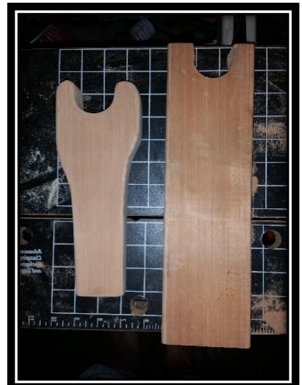
The heddle supports before and after cutting.
