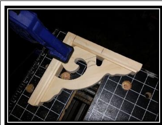
Corner trim (Cloth rod support) with cut marks
