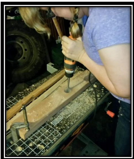
Drilling the heddle support
